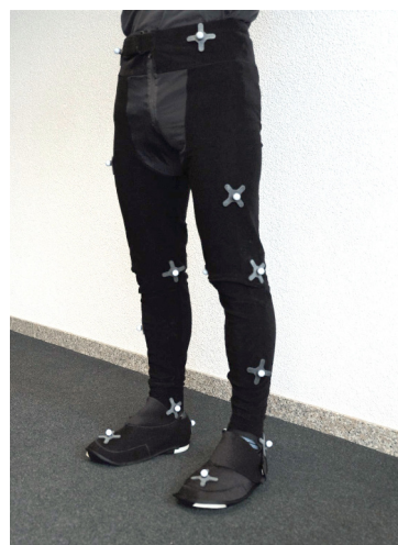
Figure 1: Left: «Plug-in Gait» Lower Body with vKAD marker placement, Right: 3D-maker (right leg: green, left leg: red, medial marker: yellow).
